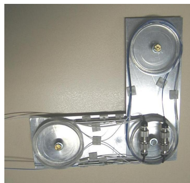
Fig. 1: Photograph of the detector showing the fibers forming the two orthogonal arms. See Fig. 2 for the schematic layout. The beam splitter and joiner are the two small stainless steel cylindrical tubes. The two FC to FC mating sleeves are physically adjacent, and the fibers can be re-connected to change from Mode A (Active detector — gravitational wave and device noise detection) to Mode B (Background — device noise measurements only). The overall dimensions are 160mm \times 160mm. The 2 \times 2 splitter and joiner each have two input and two output fibers, with one not used.
